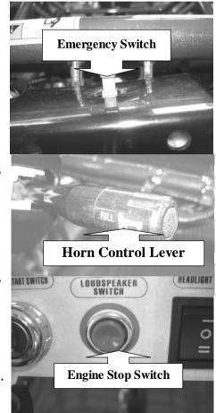
or safe switch. Press the switch, then the engine will stop. Press the switch again, then the switch will come back to normal condition.
