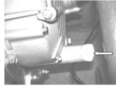
Screw off the bolt indicated in the picture, check oil level in gearbox, add it if necessary. Recommended oil: SAE15W-40 **Operation**
