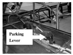
brake cable will pull the rear hydraulic disc brake to stop the vehicle, whereas loose the lever to the horizontal position to release hand brake.
