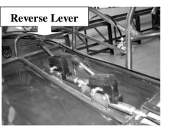
lever to N position so that you can stop the vehicle. Put the control lever to R position so that you can drive the vehicle backward.
