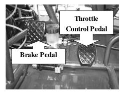
The throttle pedal is on the right side below the steering wheel and is controlled by the right foot. Step down the pedal to increase speed. When you release the foot, it will automatically return
