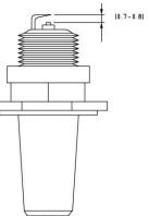
Measure the electrode gap side electrode gap (1) with a feeler.
