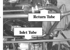
respectively; tubes are solid on the frame where close to the radiator.
