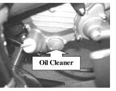
• Tilt the engine towards side of the screwed plug to drain off the used oil. Clean the filter component in the flushing oil and dry it. Clean the spring and the screwed plug. Assemble the filter component, spring and the screwed plug. Fill in 1.0-1.2L specified engine oil to the oil gauge hole on the engine and then screw in the oil gauge. Now, start the engine and run the engine for several minutes. Then, stop the engine and check the oil lever again (See Page 8.).
